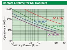
Maximal switching characteristics (DIN EN 60947-5-1)
